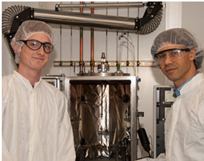
Undergraduate researcher Brian Gawlik and Dr. Paulo Ferreira, his advisor, are pictured in a cleanroom where Gawlik is preparing gold in an evaporation chamber utilizing a heat source to evaporate gold and spray it onto a carbon substrate at the top of the chamber. Read more.
